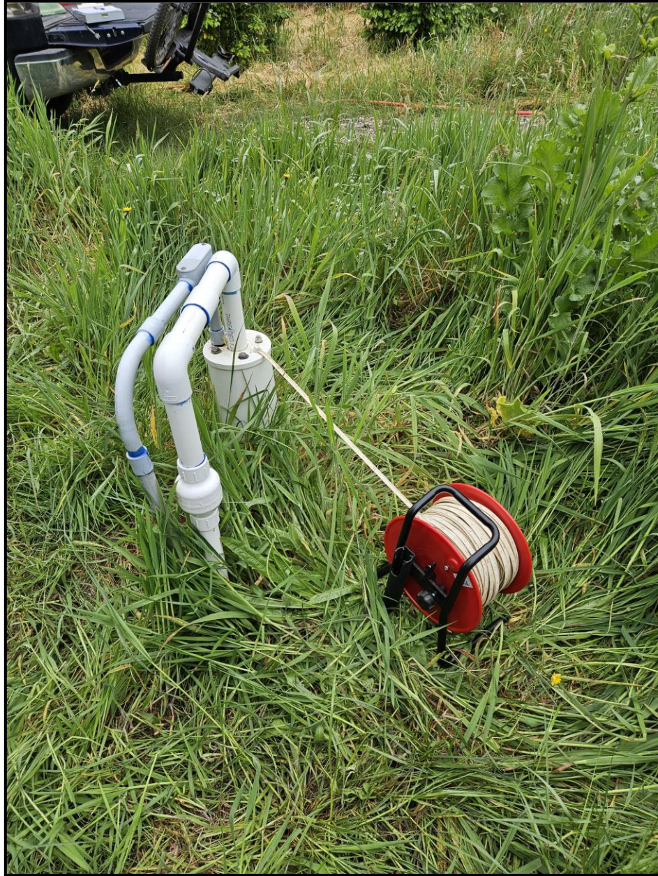
Photo 1: View of Site Well during testing.
