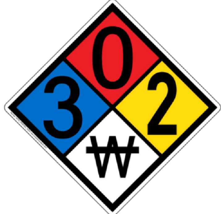
2 BATTERY FIRE SAFETY SIGN N.T.S.
