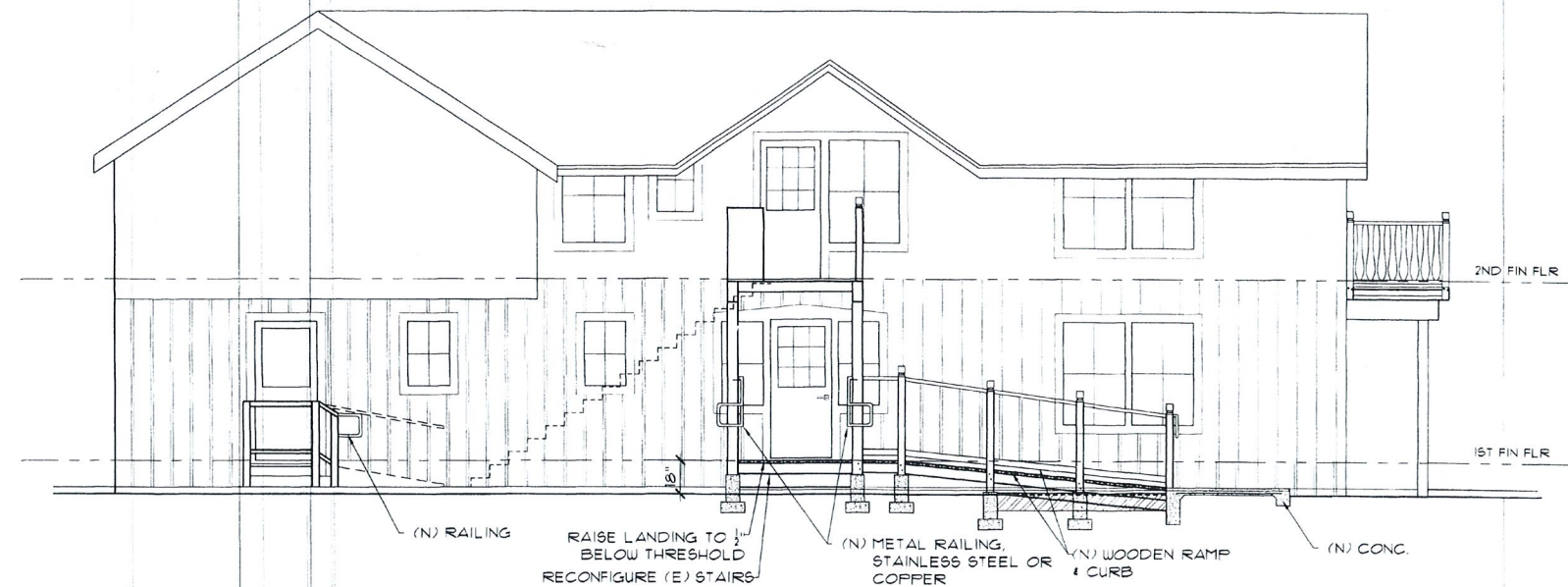
(P) WEST ELEVATION AT COURT
