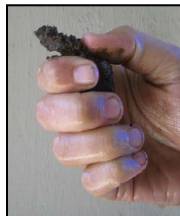
Figure 6. Squeeze soil, pushing upward into a ribbon with thumb.
