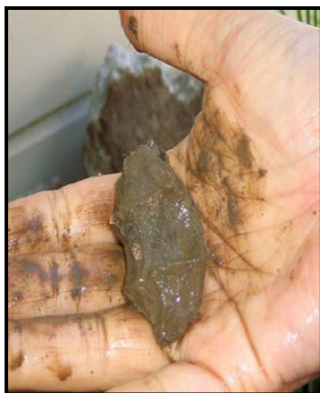
Figure 5. Prepare soil for the ribbon test by moistening and kneading.
