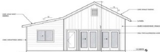
2 Existing South Elevation Scale 1/8" = 1'-0"
