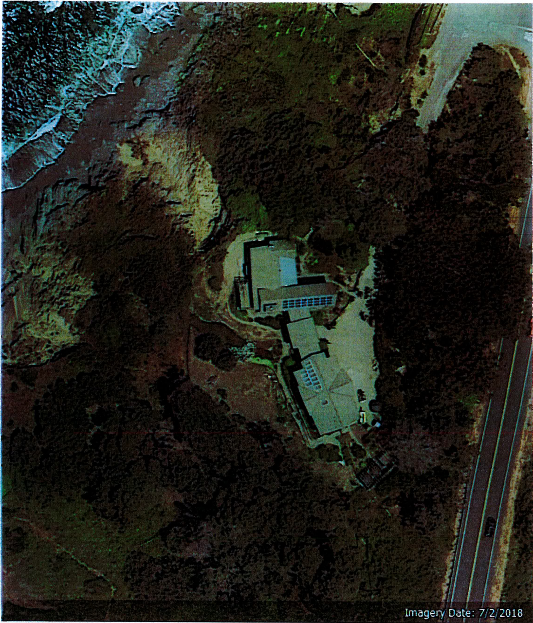
Figure 5. Google Earth aerial photo taken 7/2/2018. The slide can be seen to the northwest of the residence. This photo was taken during the residence stabilization process, the deck and lawn have been replaced, as reflected in the photos of the site below.
