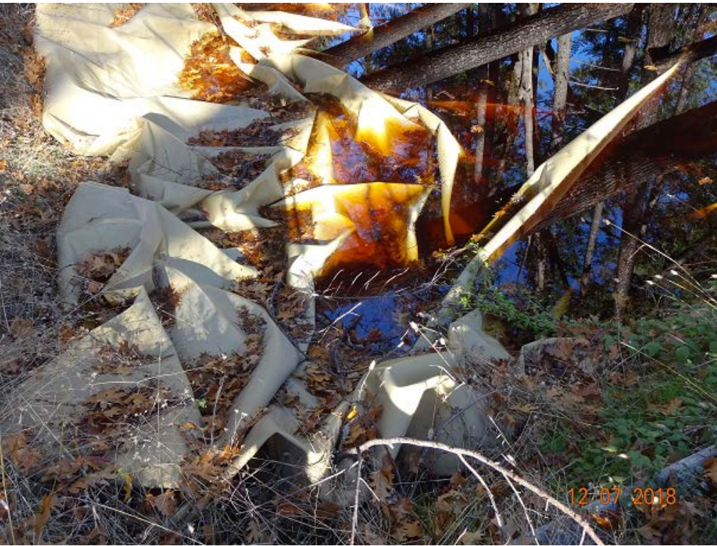
Close -up broken bladder
