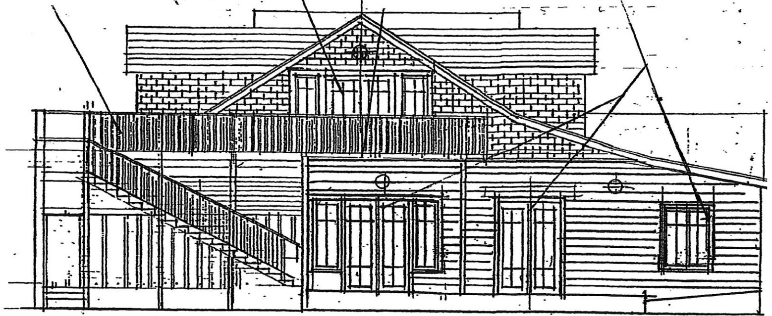
**(P) South—Stair, rebuild (E) deck, shed, (P) Garage door, (P) Replace deteriorated Wood Siding, Wood Doors & Windows.**
