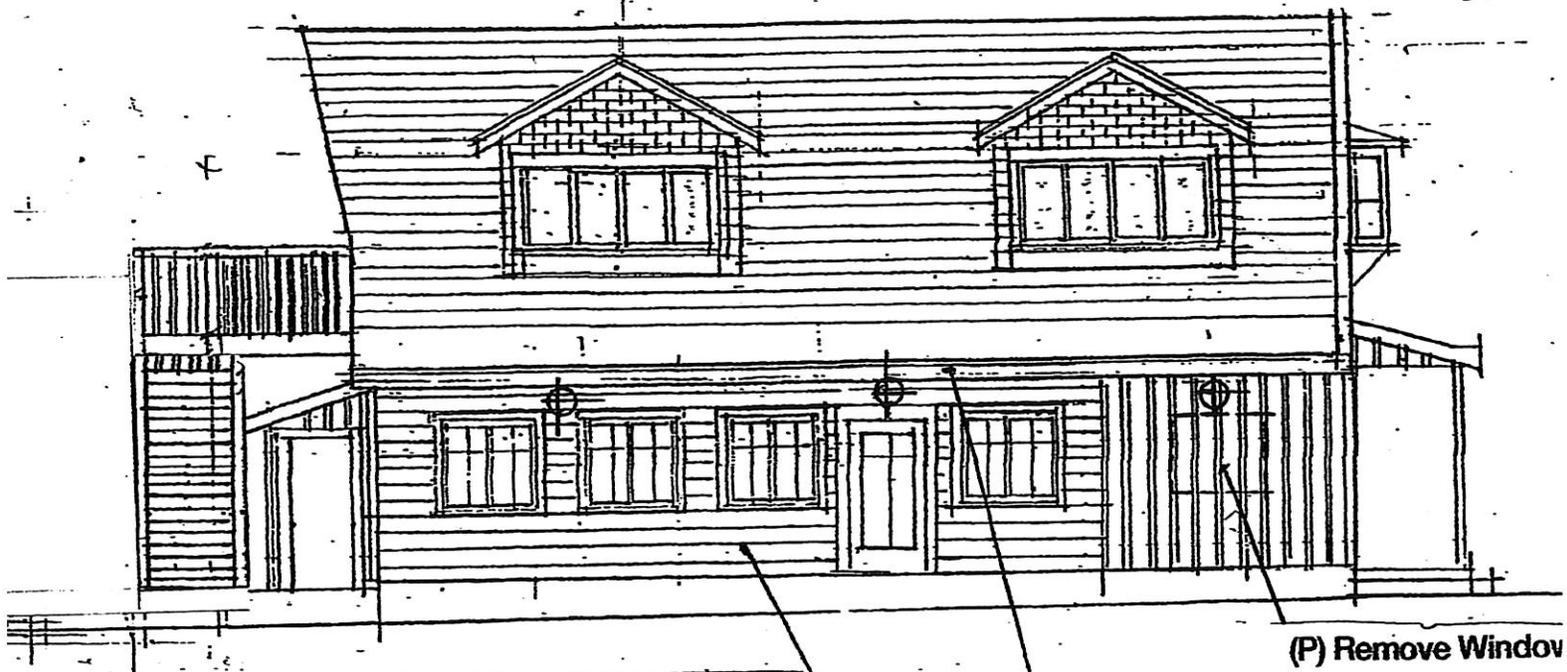
(P) East—new window wall & Raise Shed Roof to align with existing roof.
